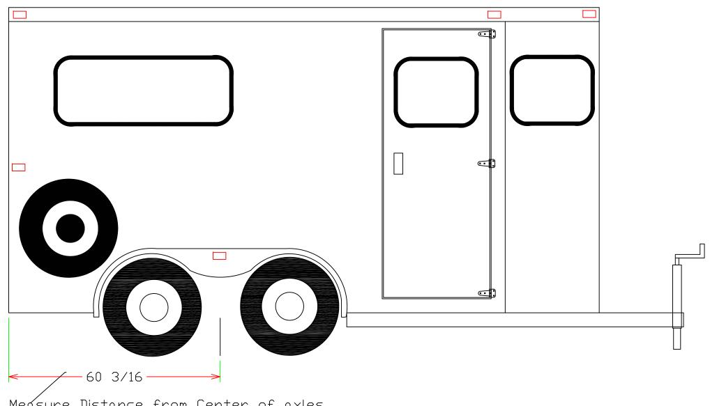
Measure Distance from Center of axles to rear of the trailer structure
