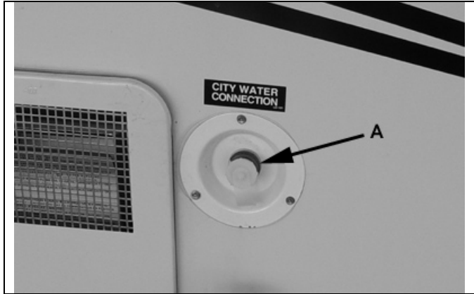
Figure 4-1 – City Water Connection
